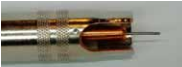
Correct positioning of contact tip.
