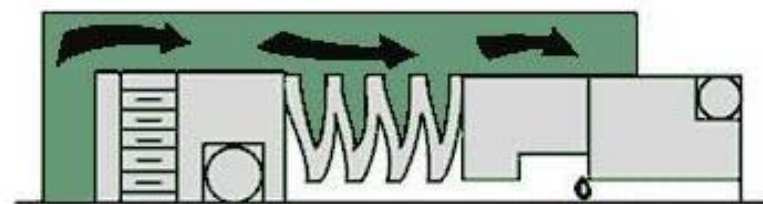
Non-pusher seal type (metal below)
