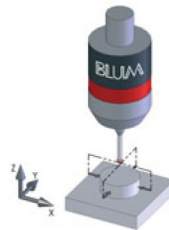
Measure an inside width or outside width
