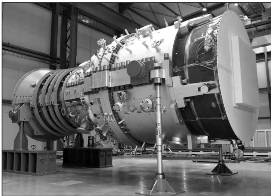
Figure 11–3 Siemens SGT5-8000H gas turbine
