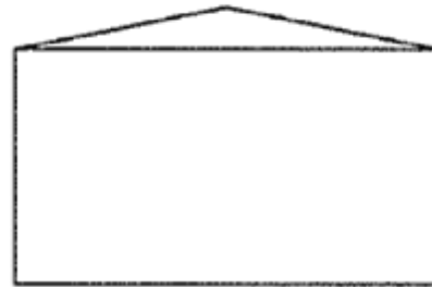
CONED FIXED ROOF TANK
