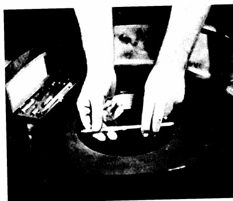
Measuring wearing ring bore with an inside micrometer.
