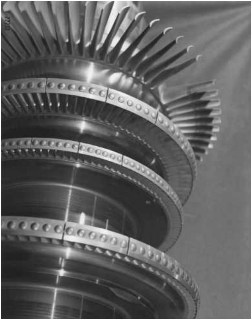
Figure 3.18. Photograph of packeted shroud bands typical of process drive turbines. (Photograph courtesy of Dresser-Rand Company.)
