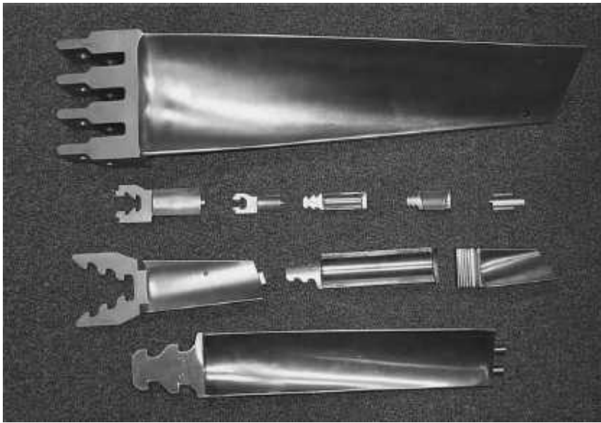
Figure 3.7. Roots commonly used in industrial steam turbines. (Photograph courtesy of Dresser-Rand Company.)
