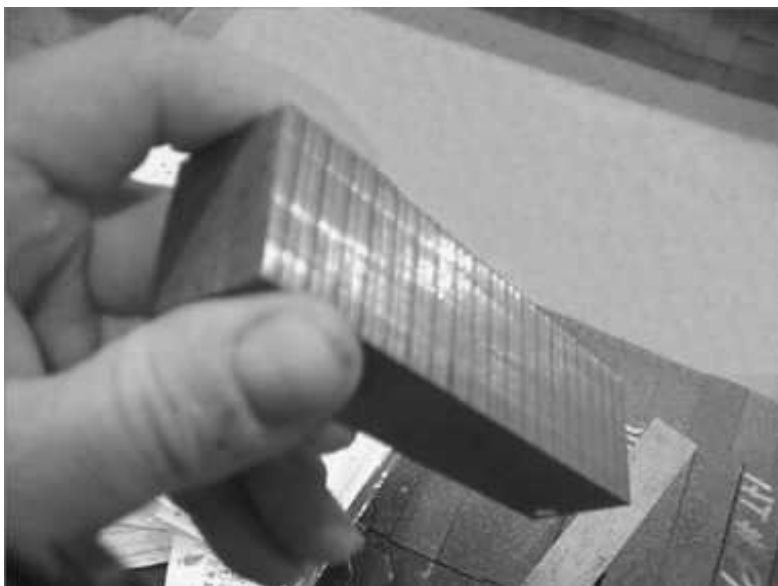
Figure 3.27. Bar stock "blank" for turbine blade. (Photograph courtesy of
