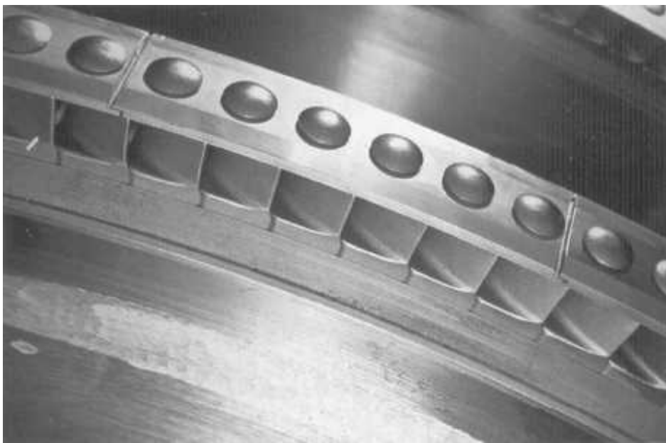
Figure 3.42. Example of correctly formed tenons. (Photograph courtesy of Dresser-Rand Company.)
