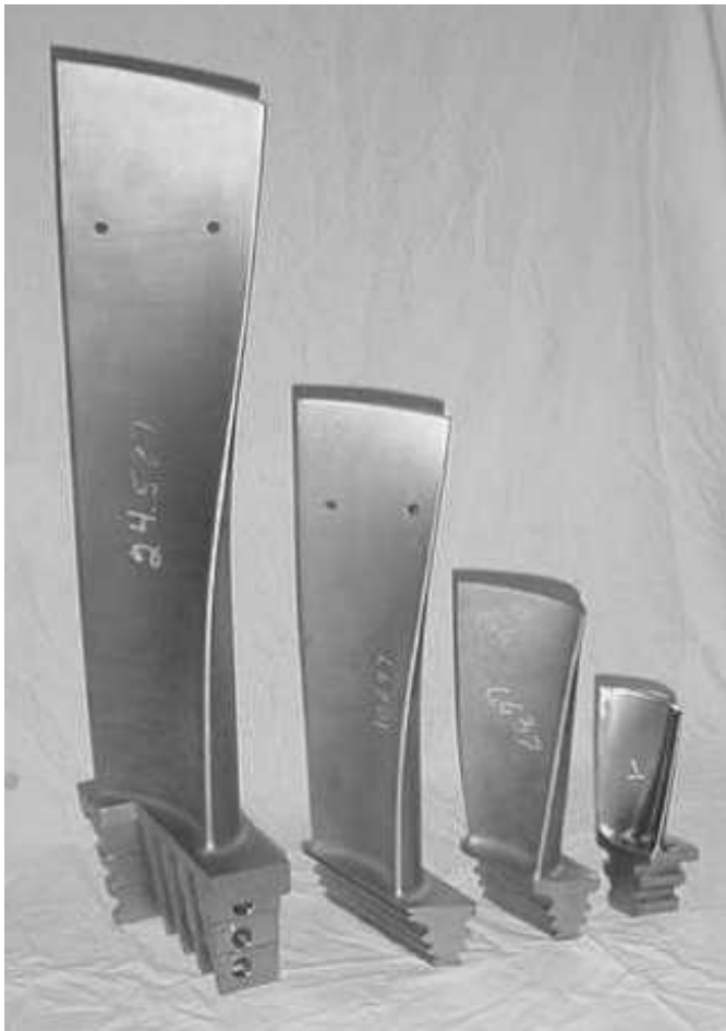
Figure 3.6. Tall blades with twisted airfoils. (Photograph courtesy of Dresser-Rand Company.)
