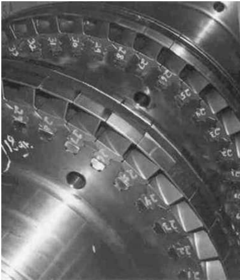
Figure 3.46. Photo of friction band shroud wire installed. (Photograph courtesy of Dresser-Rand Company.)
