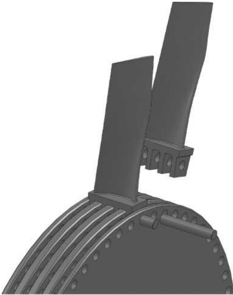
Figure 3.16. Pinned root concept—pins attach blades with one or more projecting forms that match interlacing forms on the wheel rim.
