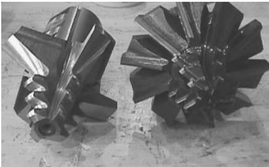
Figure 3.10. Matched dovetail root cutter set. (Photograph courtesy of Dresser-Rand Company.)
