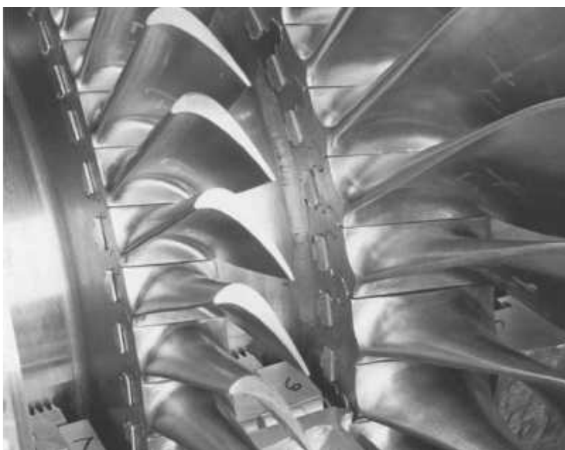
Figure 3.34. Axial roots with "dog bone" or bent-tab type of retainers. (Photograph courtesy of Dresser-Rand Company.)
