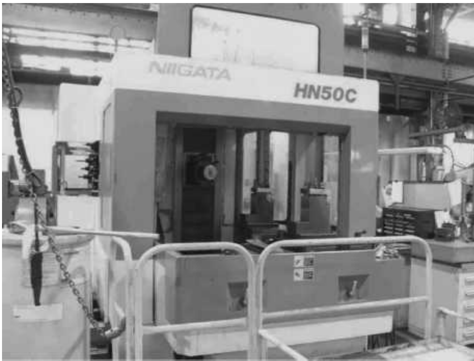
Figure 3.25. CNC machine tool for blade machining. (Photograph courtesy of Dresser-Rand Company.)
