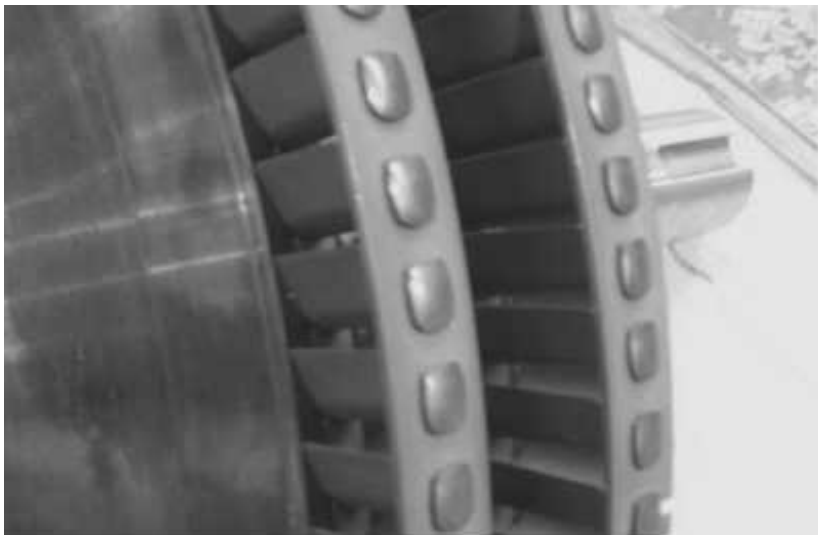
Figure 3.37. Sectional tenons after peening. Note the rectangular shape of the finished tenons. (Photograph courtesy of Dresser-Rand Company.)
