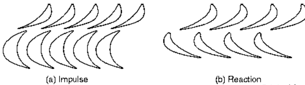
Figure 3.5. Comparison of impulse and reaction turbine cascades.
