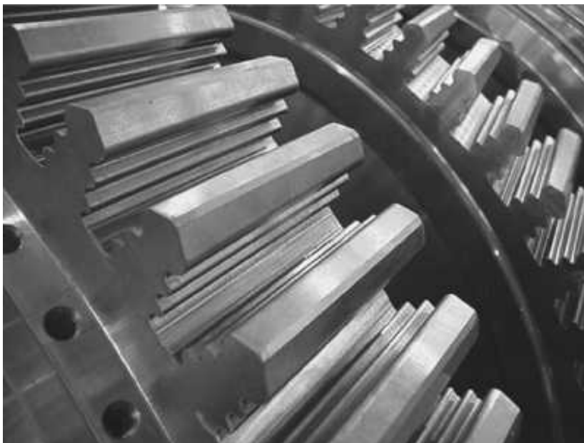
Figure 3.15. Turbine disks with milled axial roots. Note the narrow space between adjacent disks which limits the diameter of cutters and therefore the width of the root form. (Photograph courtesy of Dresser-Rand
