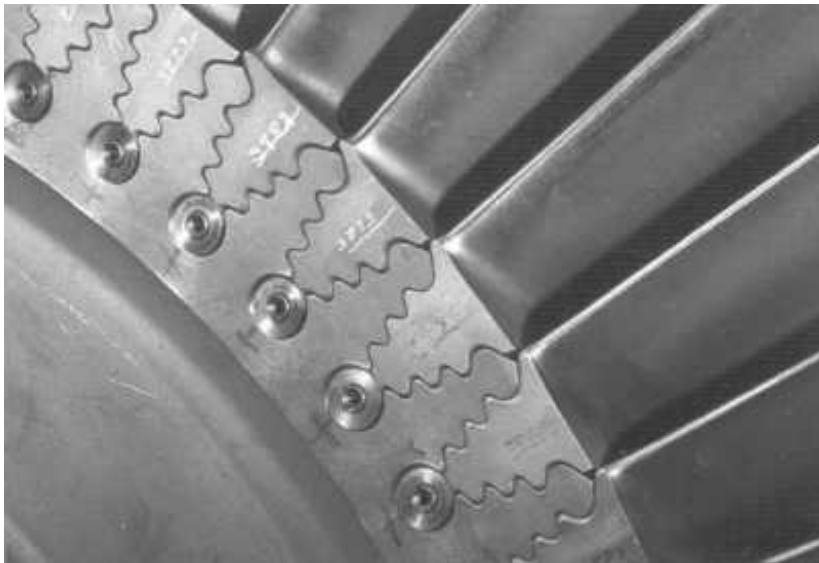
Figure 3.33. Axial roots retained with washers and rivets. (Photograph courtesy of Dresser-Rand Company.)
