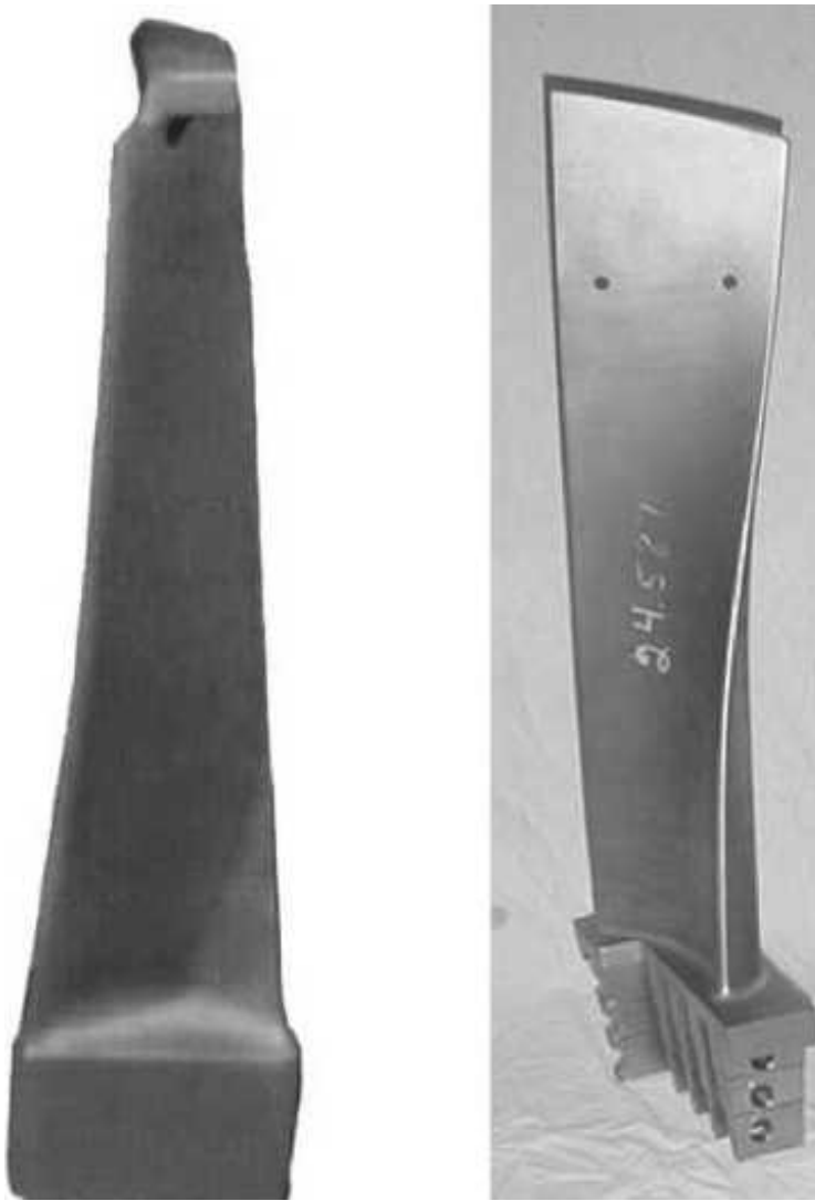
Figure 3.24. Example of envelope forging and completed blade.
