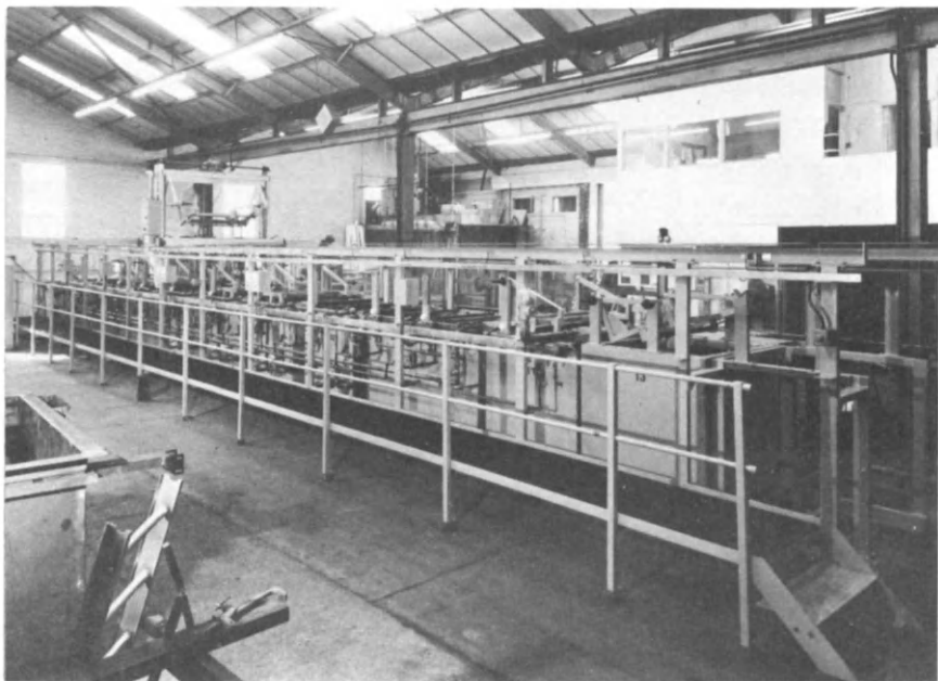
FIGURE 13. IN LINE AUTOMATIC CHROMIC ACID ANODIZING PLANT FOR DECORATIVE TREATMENT OF SMALL ARTICLES. THE CARRIER ON THE TOP RAIL CONVEYS A FLIGHT BAR OF ARTICLES THROUGH THE CLEANING, ANODIZING AND RINSING PROCESSES. THE ANODIZING VOLTAGE SEQUENCE IS ALSO AUTOMATIC. (Courtesy: Process Plant and Chemicals Ltd., Slough.)
