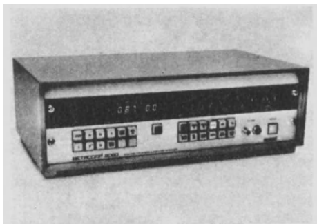
FIGURE 20. A MODERN BETA BACKSCATTER INSTRUMENT. (Courtesy: Fischer Instrumentation (G.B.) Ltd., Newbury.)
